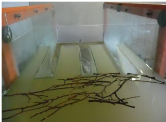
Figure 5- A view of blockage the rootstock in PKW
