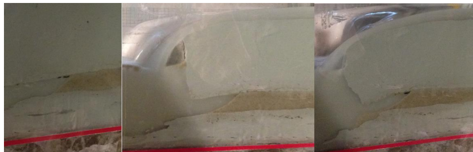
Fig. 4- Sandy layer piping in Test 5
