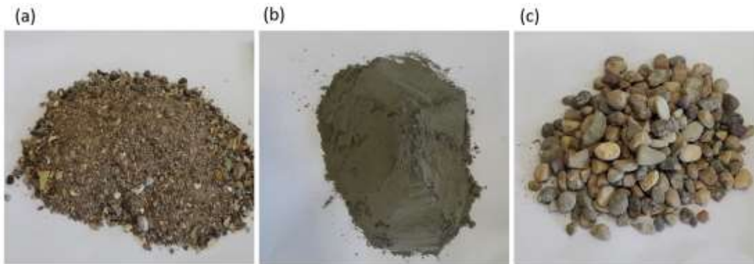
Fig. 2- Materials; (a) Fine-grained aggregates, (b) Type 2 cement, and (c) Coarse-grained aggregates
