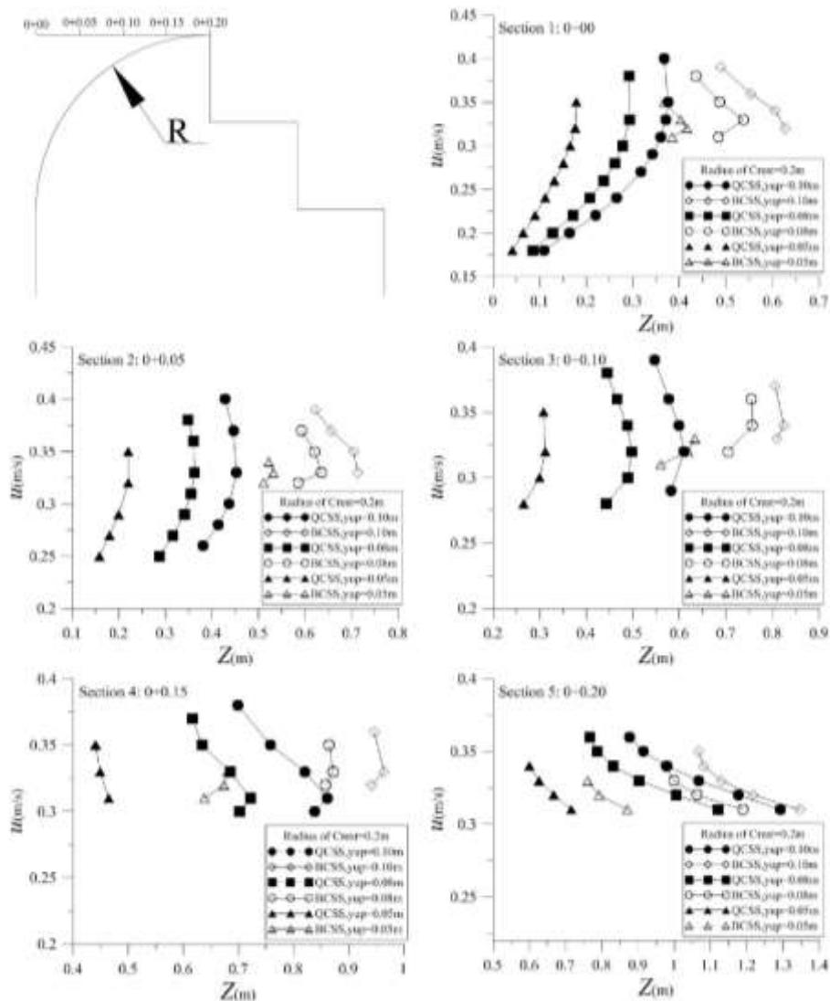
**Fig.2- Flow velocity distribution on the crest of QCSS**
