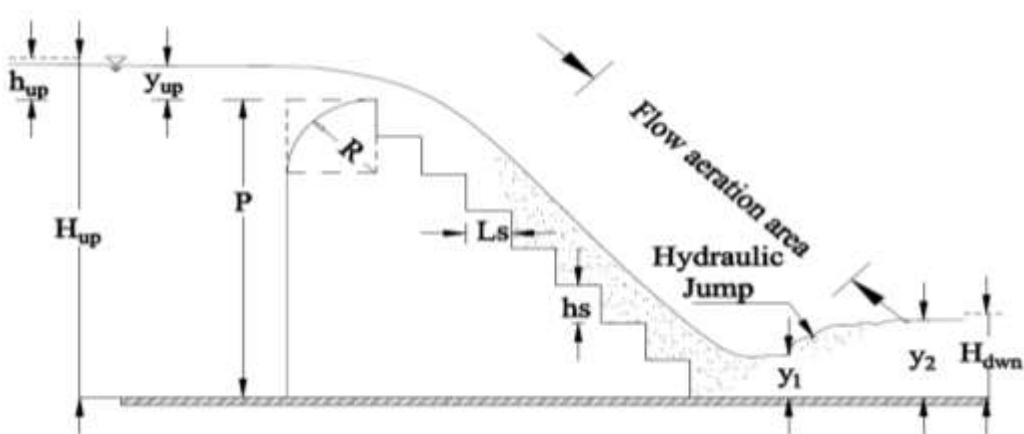
Fig. 1- The Sketch of a quarter-circular crested stepped spillway
