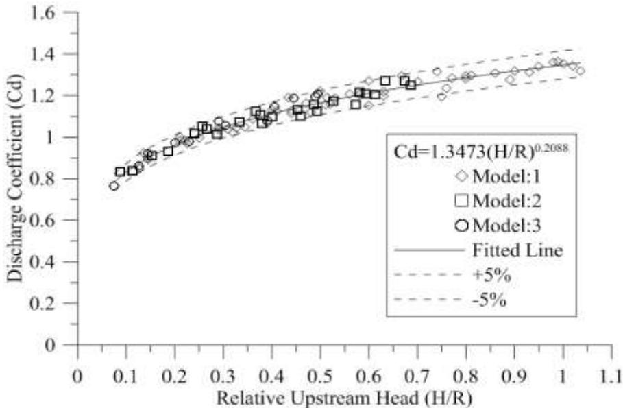
**Fig. 5- The effect of downstream slope on Cd of the QCSS versus relative upstream head**
