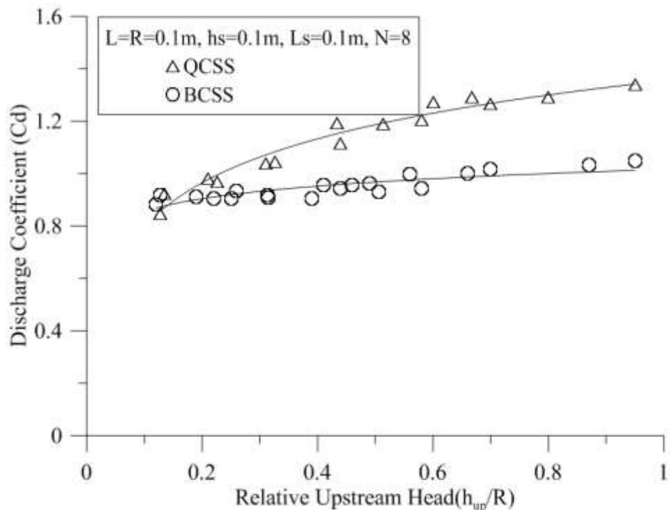
Fig. 4- The values of discharge coefficients of QCSS and BCSS
