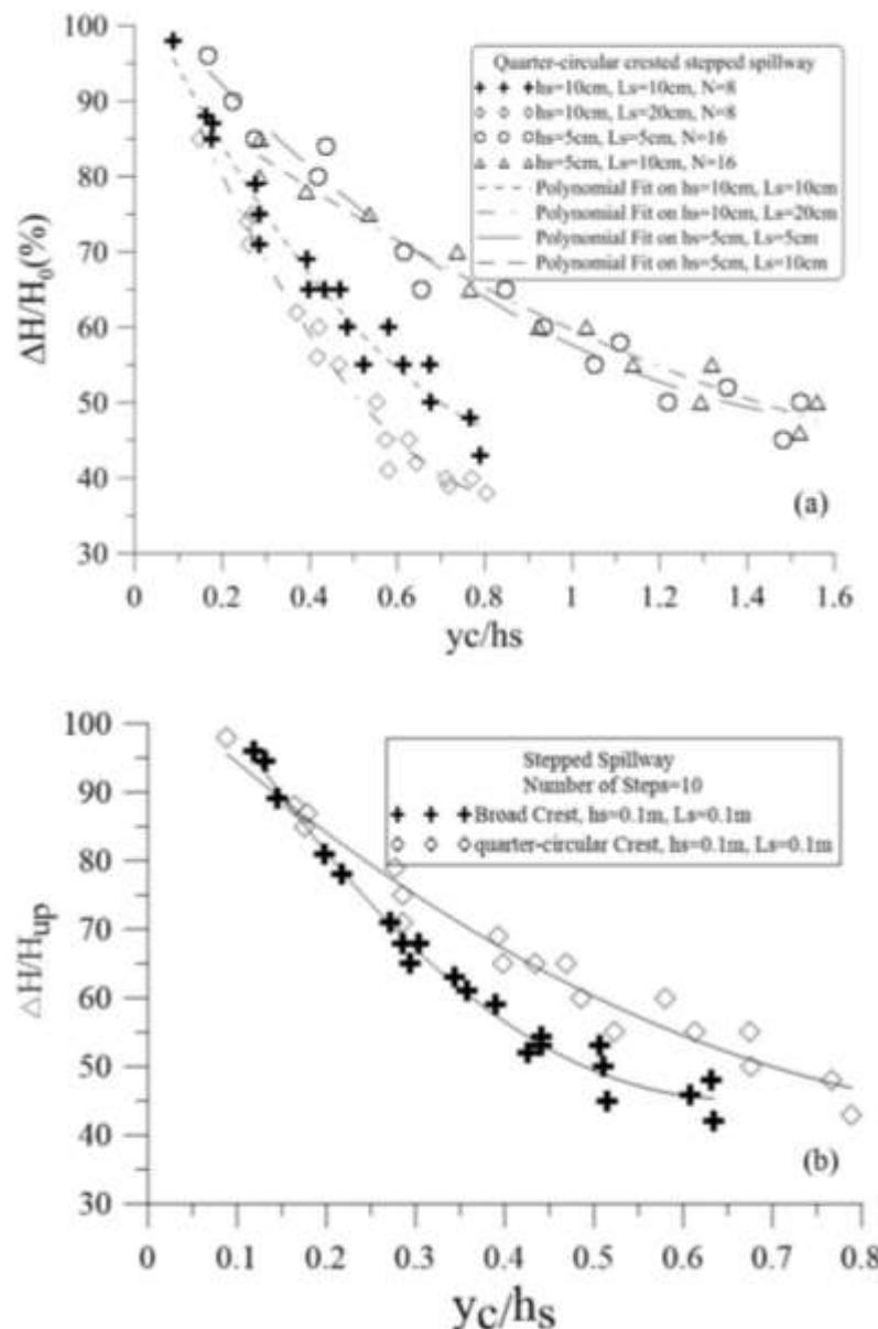
Fig. 6- The values of energy dissipation of flow on QCSS (a) and BCSS (b)
