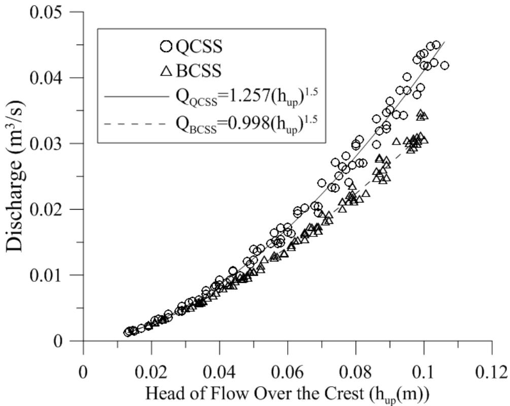
Fig. 3- The Stage-Discharge relations of BCSS and QCSS
