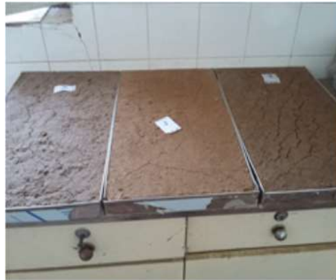
Fig. 3: Pseudo undisturbed and wetted soil sample
