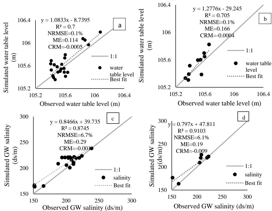
**Fig. 2- Correlation and statistical indexes between the observed and simulated water table level and GW salinity (a: Water table level calibration, b: Water table level validation, c: GW salinity calibration, d: GW salinity validation)**
