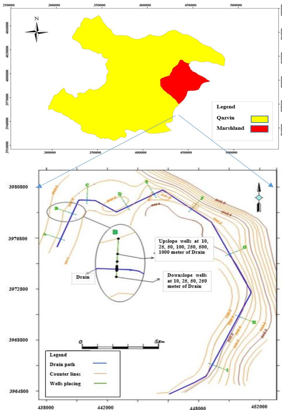
Fig. 1- Drain location, sections and observation wells
