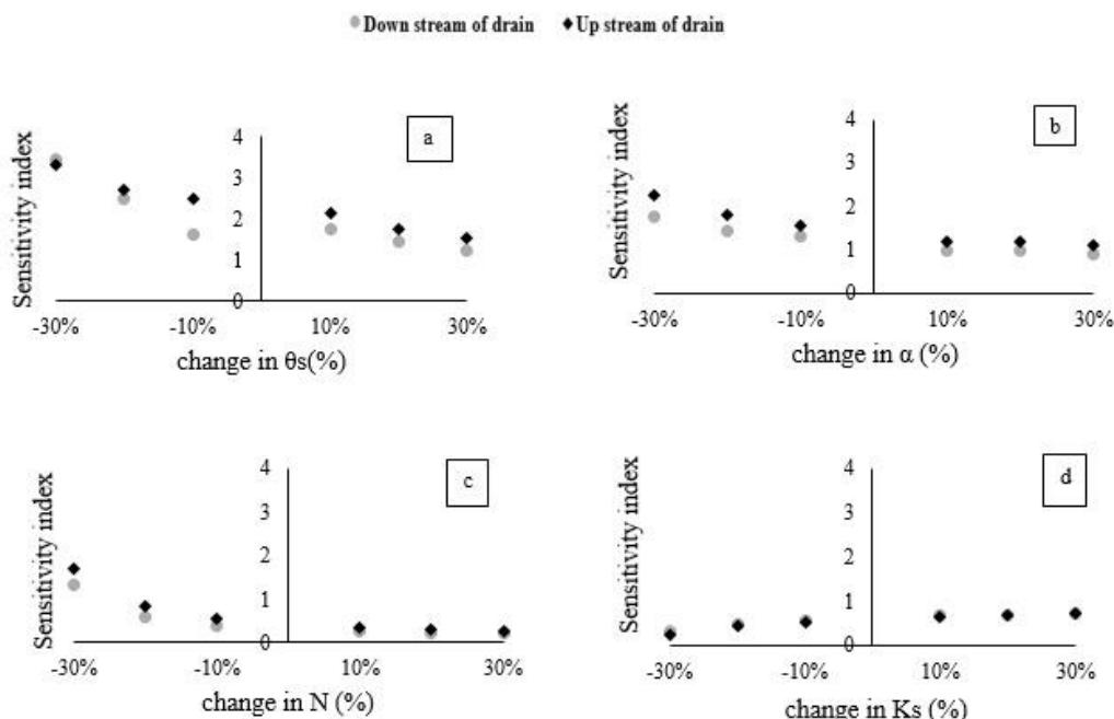
Fig. 3-Sensitivity analysis of sensitive Hydraulic parameters (a: $\theta_s$ , b: $\alpha$ , c: $N$ , d: $K_s$ )
