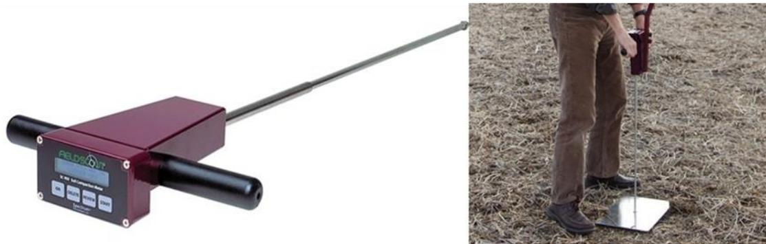
**Fig. 2- SC-900 Field Scout Digital Soil Compaction Meter (Digital Penetrometer)**
