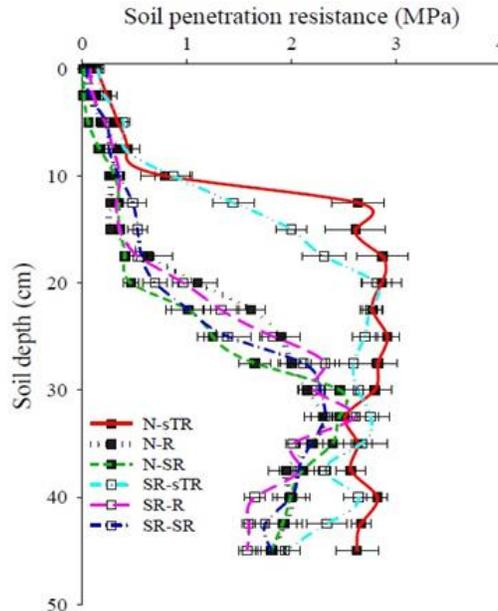
**Fig. 3-** Effect of different tillage practices on soil penetration resistance in 0–45 cm soil depth at revival stage of wheat season 2017–2018, N= no-tillage and SR= sub-soiling with rotary tillage, in the corn season; sTR= strip rotary tillage, R=rotary tillage and SR=sub-soiling with rotary tillage, in the wheat season.
