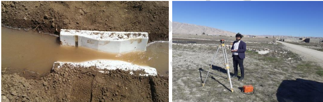
Fig. 2- WSC flume and determining the slope of the field with Nivo camera
