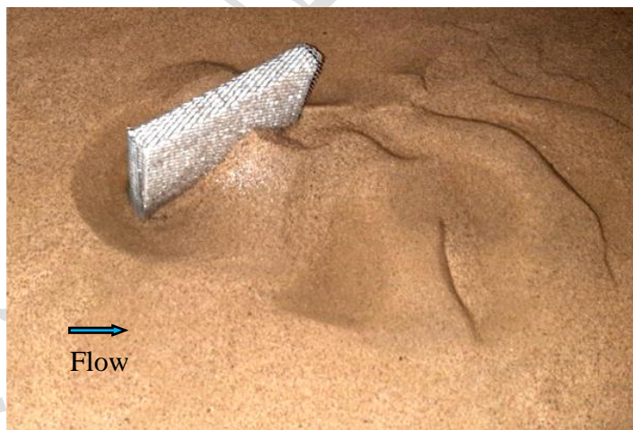
Fig.9- The position of the maximum depth of the scour hole and sedimentation bars behind the vane in test VF25 at submergence ratio T/d_0=0.5
