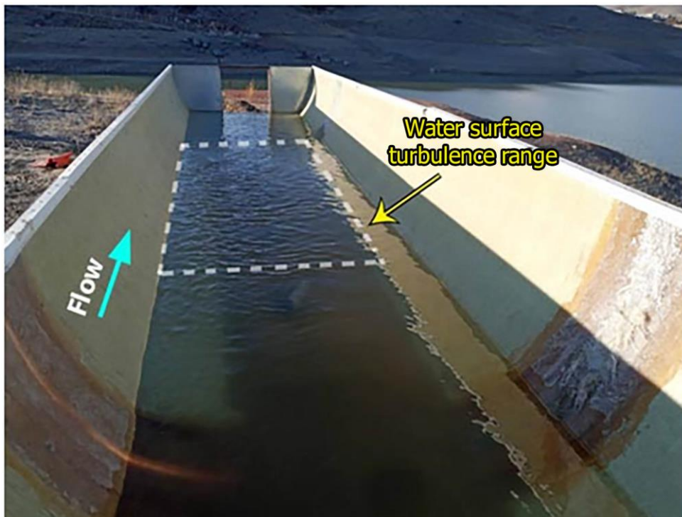
Fig.8-The effects of water surface turbulence due to shear layer eddies behind the submerged vane at submergence ratio smaller than 0.6
