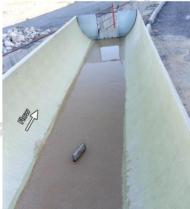
Fig. 6- view of the installation of The submerged vane on sand bed
