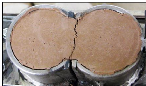
Fig. 2- Failure of a typical samples prepared with 20% moisture content and \gamma_d = 1.62 \frac{gr}{cm^3} ,
