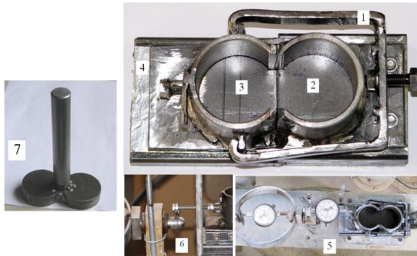
Fig. 1- Different parts of the tensile device and their connection to the direct shear apparatus lever: 1) Holding clamp, 2) Fixed mold, 3) Movable mold, 4) Horizontal platform, 5) Placement on the direct shear apparatus platform, 6) Connection of the movable mold to the force application lever, 7) Rammer for compaction of specimens
