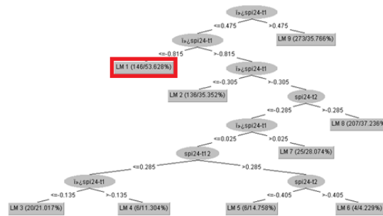
Fig. 6- Diagram of the M5 model tree with nine linear regression models at the leaves.
