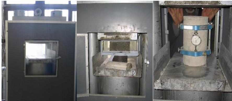
Fig. 2- From right to left, Machines for measuring compressive strength, tensile strength and elasticity
