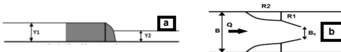
Fig. 3– (a) Longitudinal profile of the flow through the Lopac gate, (b) View from above the stream passing through the Lopac gate
